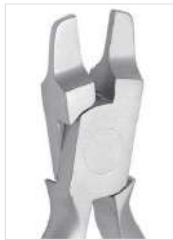
Tweed Arch Forming (0.9 mm thick) Cat.No. AC-135
