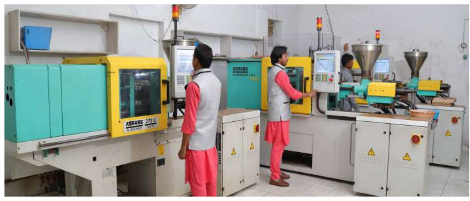
Metal Injection Moulding (MIM) using German Machines
